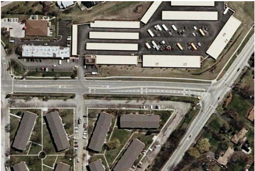
BUTTERFIELD ROAD BUILT FOR FUTURE EXPANSION TO DUAL LEFT TURNS.
